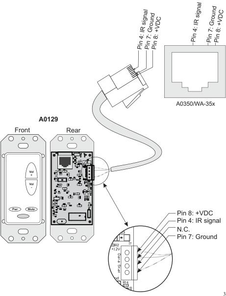
**Using the A0505 remote control..** designed to control your A0350, WA-35x. (Download IR codes at: www.channelvision.com and www.remotecentral.com)
